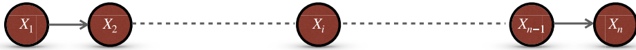
Figure 14. An inhomogeneous Markov chain consists of X = \{X_1, X_2, \dots, X_n\} with p(x) = \prod_{i=1}^n p(x_i|x_{i-1}) .
